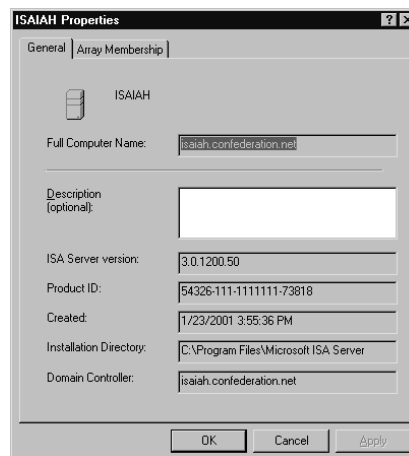
Figure 24.22 Access the Properties Sheet for Each Array Member through the Computers Folder
