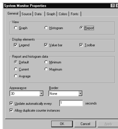
Figure 25.4 The System Monitor Tool's Appearance Can Be Customized Using the Properties Sheet
