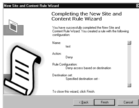
Figure 24.29 The ISA Wizards Allow You to Check the Information Entered for Accuracy Before You Click Finish
