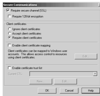
Figure 27.69 Forcing a Secure Channel to the Web Site
