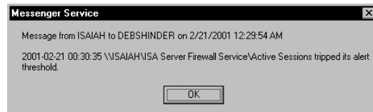
Figure 25.12 A Network Message Is Sent to the Specified Account When the Alert Is Triggered
